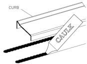
NOTE: IMPROPER CAULKING WILL RESULT IN LEAKS.
