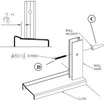
FOR TILE OR MARBLE WALL9, DRILL 91X 3/16" DIAMETER HOLES AND INSERT PLASTIC WALL ANCHORS [C]. ATTACHMENTS TO FIBERGLASS OR ACRYLIC UNITS CAN BE MADE IN TWO WAYS. IF REIN- FORCEMENT IS BUILT INTO THE WALL, DRILL 91X 1/8" DIAMETER HOLES AND INSTALL MOUNTING SCREWS. IF WALLS ARE NOT REINFORCED DRILL 3/16" HOLES AND INSTALL PLASTIC WALL ANCHORS OR MOLLY BOLTS (MOLLY BOLTS NOT SUPPLIED).
