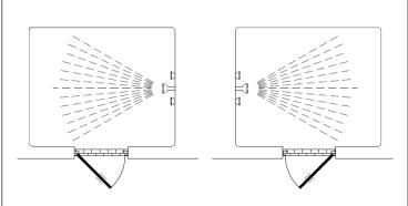
I. THE MODEL 30C FRAMELESS CONTINUOUS HINGE DOOR IS REVERSIBLE AND MAY BE INSTALLED PIVOT-RIGHT OR PIVOT-LEFT. USE THIS DIAGRAM TO DETERMINE THE CORRECT POSITION FOR YOUR INSTALLATION. FOR MAXIMUM WATERPROOFING THE PIVOT JAMB SHOULD ALWAYS BE OPPOSITE THE SHOWER HEAD. THESES INSTRUCTIONS DEPICT A PIVOT-RIGHT INSTALLATION. DOOR MUST ALWAYS OPEN OUTWARD.
