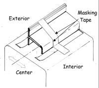
3. REMOVE THE PARTS AND DRILL 1/8" HOLES APPROXIMATELY I INCH DEEP IN EACH WALL IN THE MARKED LOCATIONS. IN TILE OR MARBLE WALLS, IT MAY BE NECESSARY TO DRILL 3/16" HOLES AND INSERT THE
