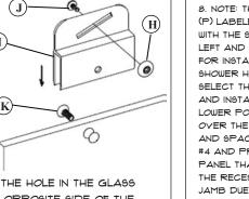
SCREW (K) THROUGH THE BRACKET, THE HOLE IN THE GLASS DOOR PANEL AND THREAD INTO THE OPPOSITE SIDE OF THE BRACKET. TIGHTEN SECURELY. REPEAT THIS PROCEDURE FOR THE REMAINING THREE BRACKETS.
