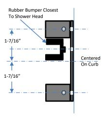
3. If using the wall plugs, drill six ¼" diameter holes in the positions marked. Attach the brackets and rubber bumpers with the screws provided. If not using the plugs, drill 3/16" diameter holes thru the substrate and allow the screws to tap into the stud.
