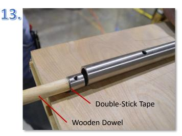
Use a ½" wooden dowel rod and double stick tape to insert the Threaded Retainer inside the Header. Slide into position with the threaded hole lining up with the drilled holes in the header.
