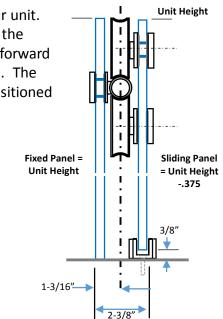
On the wall away from the shower head, make a mark 3-1/2" below the unit height and directly on the centerline. This is the location of the header.
