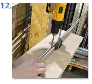
Check the centerline dimension of the two holes in the Fixed Panel and drill a second 3/8" diameter hole spaced this exact dimension from the first hole. *Note: It is important that both holes are in alignment. See illustration.*
