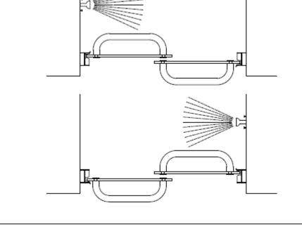
with the shower head on the left and 4 bumpers labeled "R" for installations with the shower head on the right. Select the correct bumpers and install by pressing the lower portion of the "keyway" over the head of the screw and spacers installed in step **#4** and pressing down.
