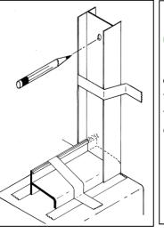
Replace one wall jamb and attach to the wall by pressing a nylon spacer [E] over two #8 x 1-1/2" truss head screws [D] and insert through the top and bottom holes. Install a third screw in the center hole. Check for plumb before tightening the screws. Repeat for the other wall jamb.
