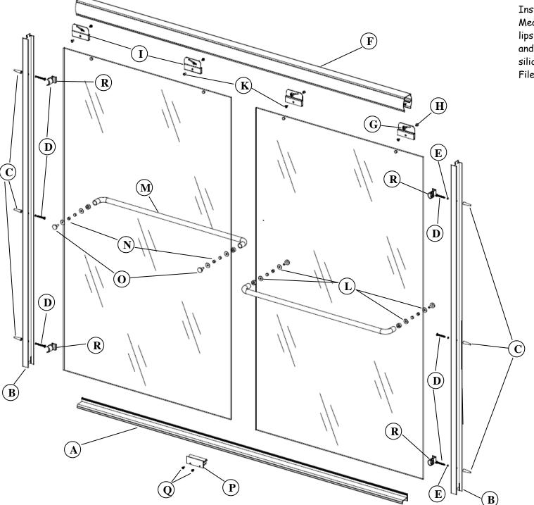
Installation Tools Required: Tape Measure, Masking Tape, Level, #2 Phillips Screwdriver, Drill with 1/8", 7/64" and 3/16" bits, hacksaw, pencil, clear silicone caulking. Optional: Miter Box, File and Center-Punch.
