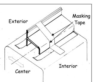
Remove the parts and drill 1/8" holes approximately 1 inch deep in each wall in the marked locations. In tile or marble walls, it may be necessary to drill 3/16" holes and insert the plastic wall plugs [C]. Using a caulking
