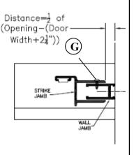
Inside the enclosure, drill two 1/8" holes through the strike jamb [E] and into the wall jamb [B] 3/8" to 3/4" from the wall and approximately 1" vertically from each end of the strike jamb. Drill a third hole centered between the first two. Enlarge the three holes in the strike jamb with a 3/16" drill for clearance on the self-tapping screws. Attach the strike jamb with three #6  $\times$  3/8" pan head screws [G].
