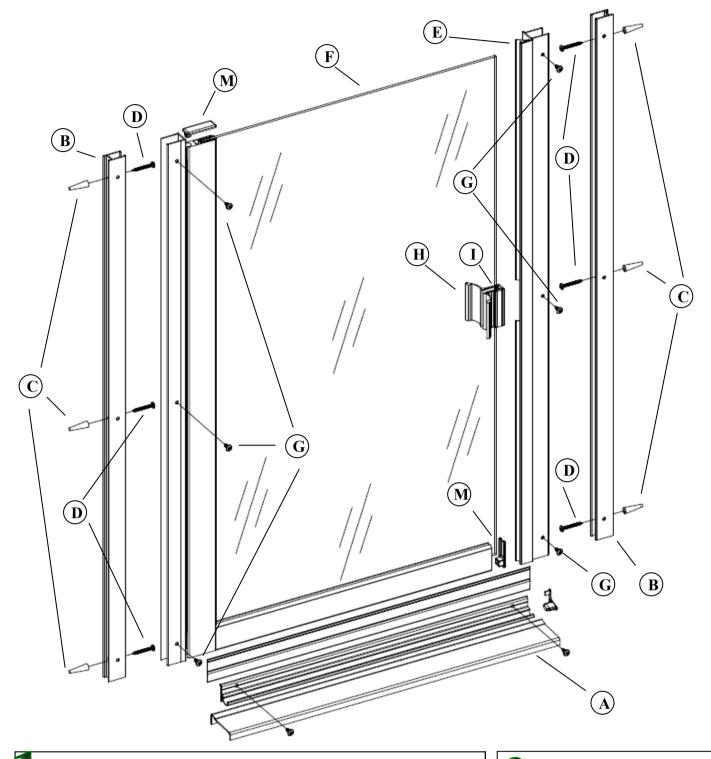
Installation Tools Required: Tape Measure, Masking Tape, Level, #2 Phillips Screwdriver, Drill with 1/8", 7/64" and 3/16" bits, hacksaw, pencil, clear silicone caulking. Optional: Miter Box, File and Center-Punch.
