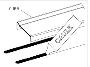
NOTE: Improper caulking will result in leaks.
