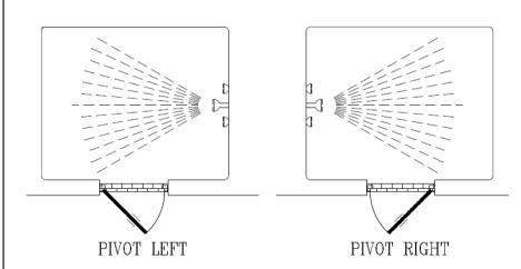
NOTE: Obscure glass doors should be installed with the rough surface of the glass to the exterior of the unit. Make sure the glass is driven into the hinge rail a full 3/4".
