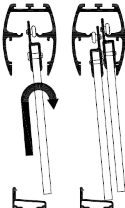
**9** Locate a bottom guide [R] in the center of the track with the interior panel positioned as shown. Drill a mounting hole in the track with a 7/64" bit using the hole in the guide and the V-groove in the track to locate properly. Attach with a #6 x 3/8" pan head screw [S]. Optionally you may also locate a guide in the center of each door opening using the same procedure.
